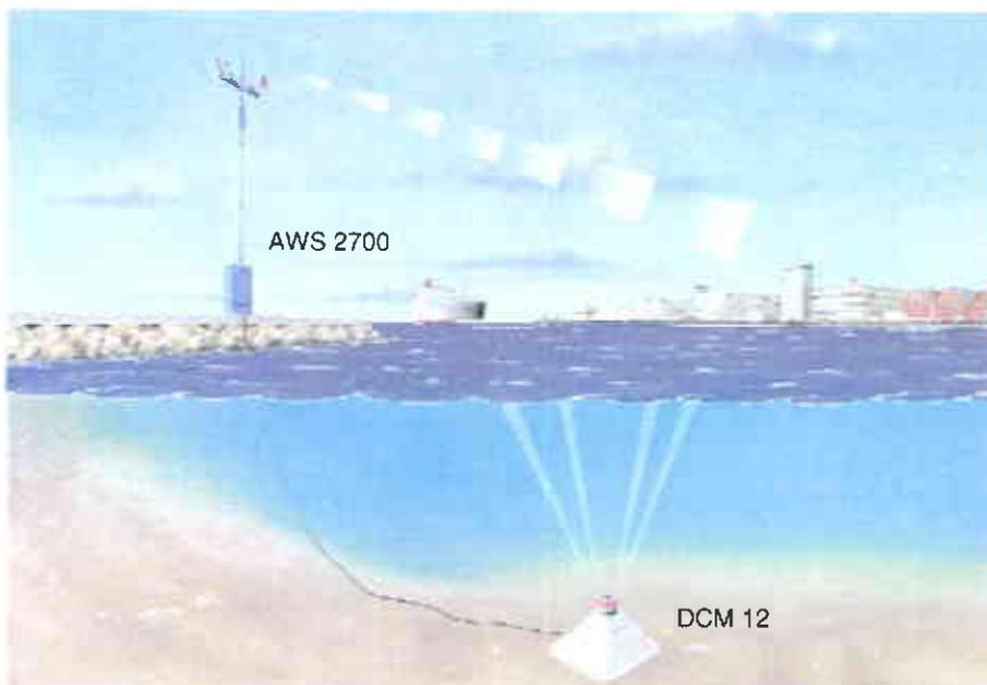
The Port Environment Information System from Aanderaa is developed to aid ship navigation in harbors, canals, rivers, channels and other narrow waterways.
