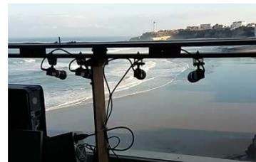
$$\eta(t) = \eta_{\text{tide}} + \eta_{\text{surge}} + \underbrace{\eta_{\text{wave set-up}} + S_{\text{swash}}(t)}_{\text{Wave Run-up}}$$
