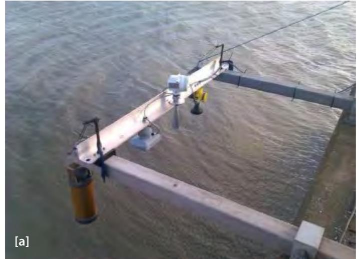
**Figure 1 [a].** The test frame at Holyhead holding (left to right) an OTT Kalesto that was not part of the test, an OTT RLS, a Waterlog H-3611 and a VEGAPULS-61. In this photograph the gauges are measuring the sea surface.
