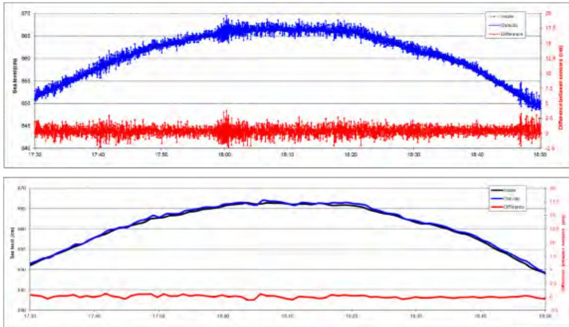
**Figure 2.** Comparison at Brest tide gauge between radar measurements inside and outside the stilling well using 1s data (above – black curve is hidden under the noisy blue one) and 15s averaged data (below)
