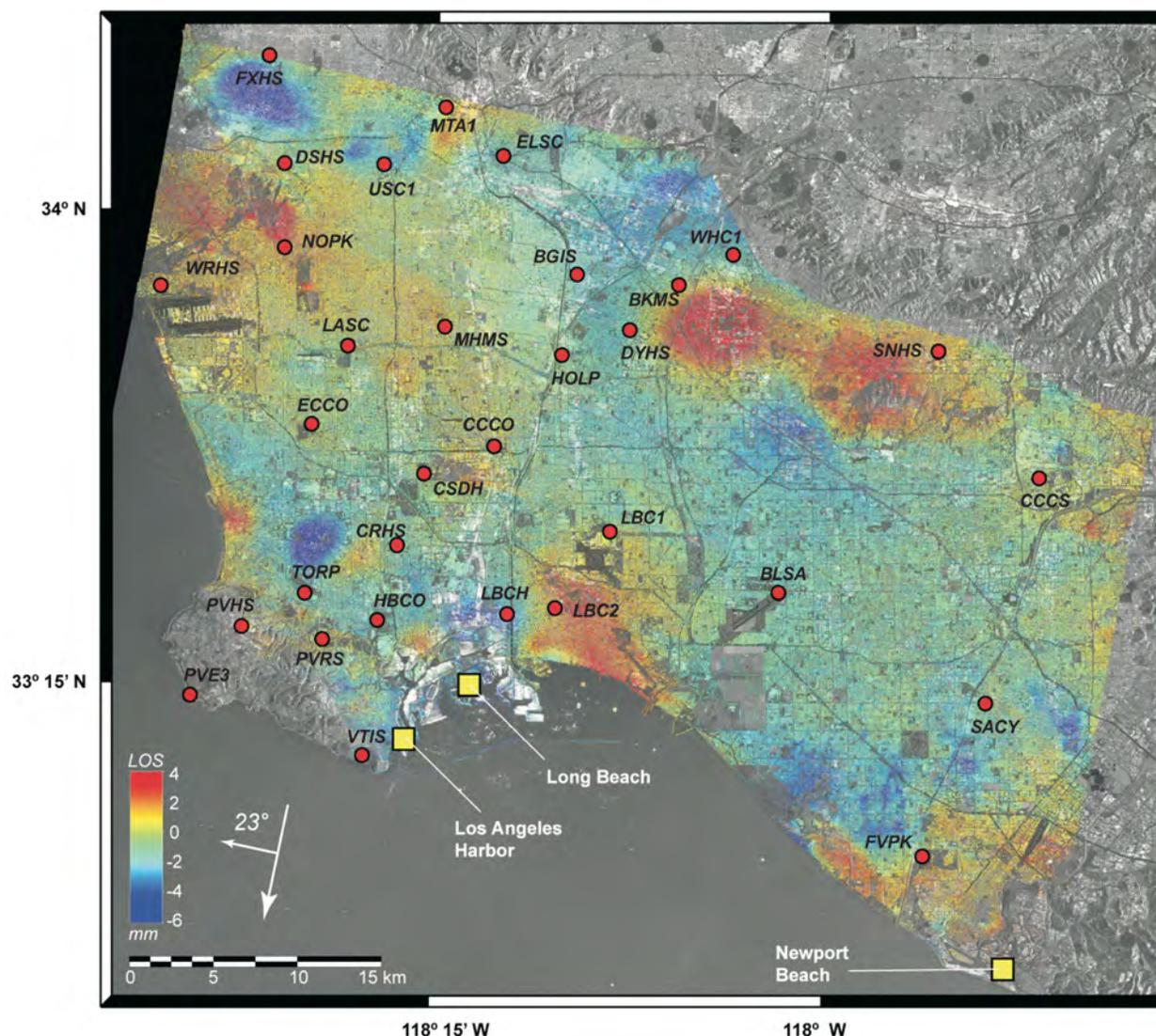
**Figure 6.5** Linear line-of-sight (LoS) velocity, which for present purposes can be regarded as the rate of vertical land movement, for the period 1992–2000 using ERS-1 descending passes across the Los Angeles basin. Continuous GNSS stations used in the analysis (red circles) and tide gauge stations (yellow squares) are shown. The legend arrow shows ERS LoS azimuth and inclination (23°). From Brooks et al. (2007).
