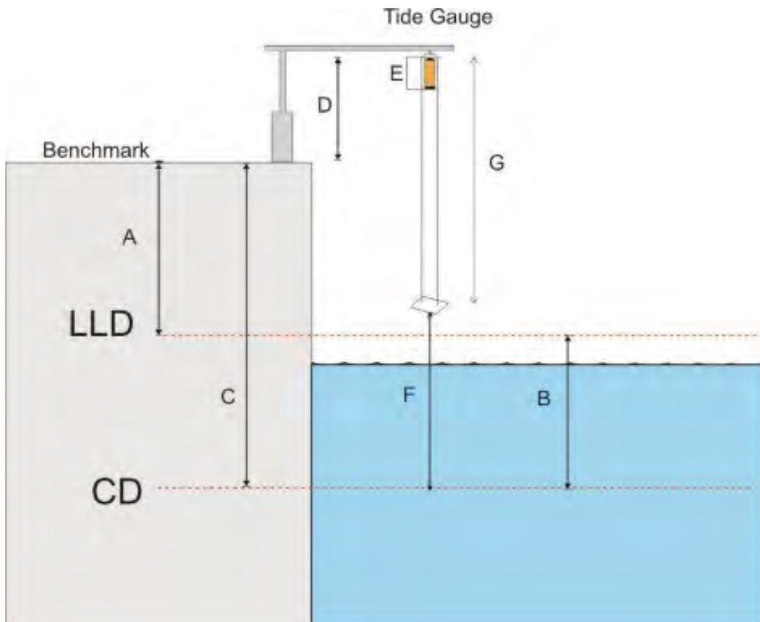
We can define this height above CD to be  $Y = A + D - E - 0.005 + B$  and the tide gauge, if correctly calibrated, should now be reading  $Y - (G - E)$ .
