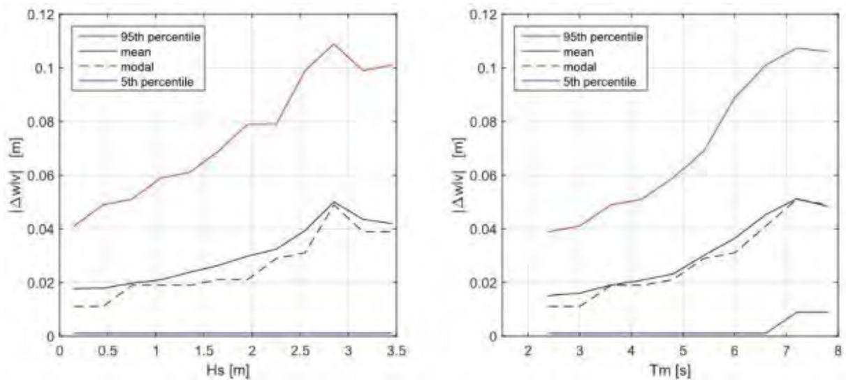
**Figure 13.** Influence of sea state at the lighthouse “Alte Weser” on the deviation between water level measurements with a single radar sensor and a float in a stilling well: effect of significant wave height (left) and effect of mean wave period (right)
