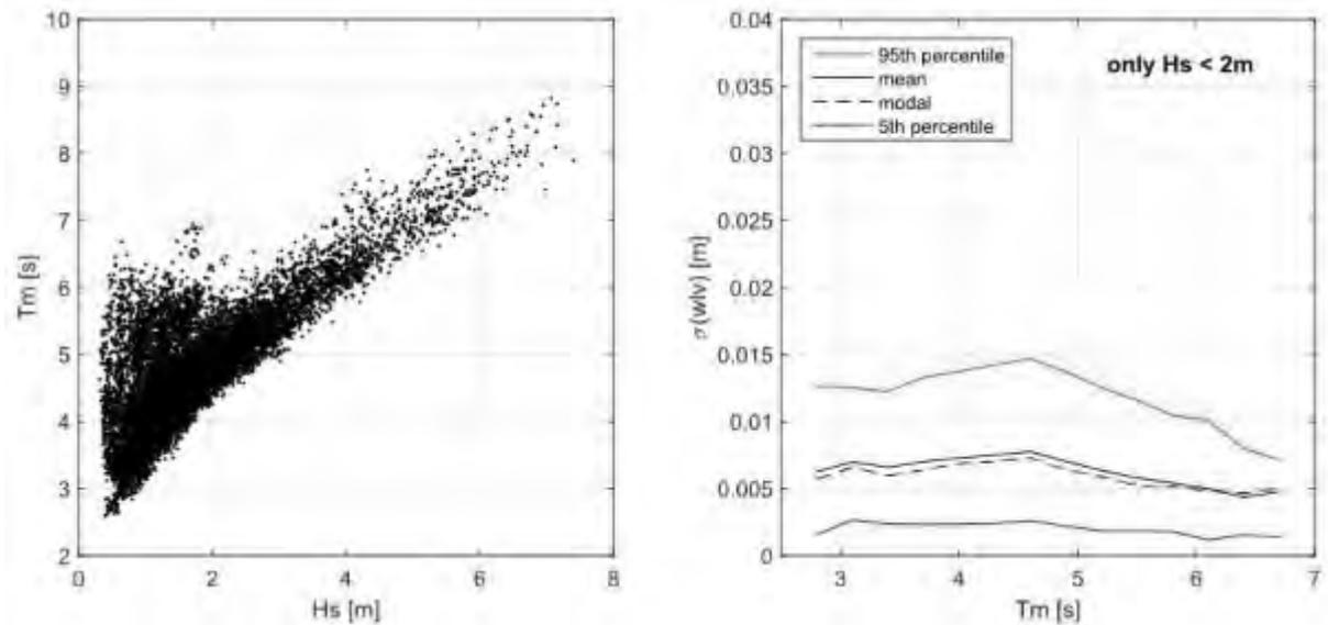
**Figure 9.** Correlation of significant wave height and mean wave period at FINO 1 (left), influence of mean wave period on the standard deviation of water level measurements with 4 radars for significant wave heights < 2 m (right).
