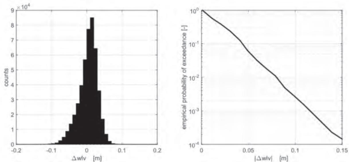
**Figure 12.** Histogram of deviations of 1 min values of water levels measured with a single radar sensor and a float in a stilling well at the lighthouse “Alte Weser” (left) and empirical probability of exceedance of the absolute deviation (right).
