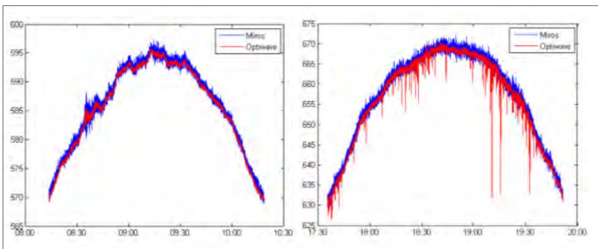
**Figure 9.** Zoom on sea level measurements of open air sensors Miros (blue) and Optiwave (red). These pictures show very good correlation (left), but also spikes on Optiwave data (right).
