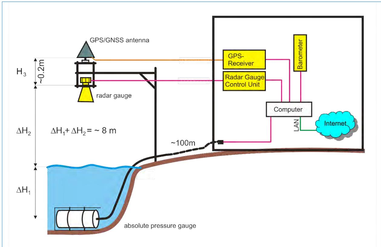
**Figure 3** Overview of the complete gauge system in GARS O'Higgins, Antarctica.
