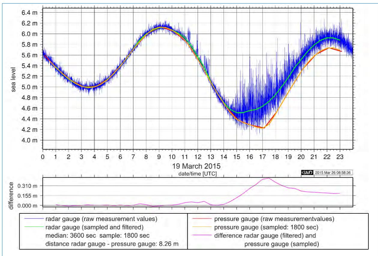
**Figure 10** Example for time series of the pressure gauge and the radar gauge in GARS O'Higgins. You can see a vertical displacement of the pressure gauge. The height position of the radar gauge is GPS controlled. In this case, the reason for the displacement of the pressure gauge could be determined, a small iceberg that scraped over the bottom and took the pressure gauge a little bit with it.
