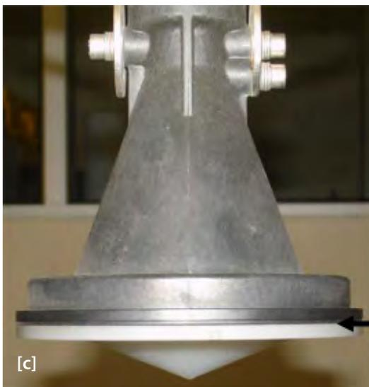
Figure 2. Reference marks on each gauge that we assumed initially would correspond to zero range.
