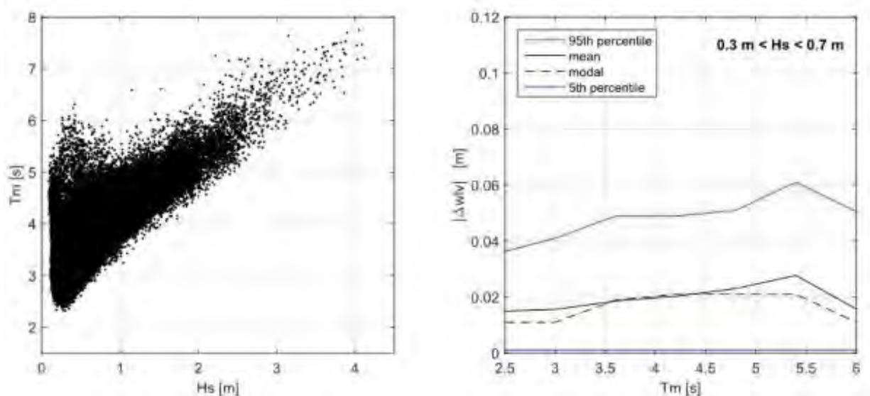
**Figure 14.** Correlation of significant wave height and mean wave period at lighthouse “Alte Weser” (left), influence of mean wave period on the standard deviation of water level measurements with 4 radars for significant wave heights with  $0.3 \text{ m} < H_s < 0.7 \text{ m}$  (right).
