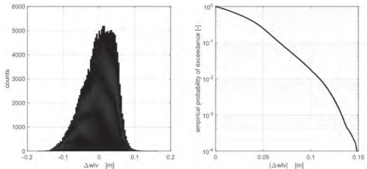
**Figure 10.** Histogram of deviations of 1 min values of water level measurements measured with radar array and float in a stilling well near Borkum (left) and empirical probability of exceedance of the absolute deviation (right).
