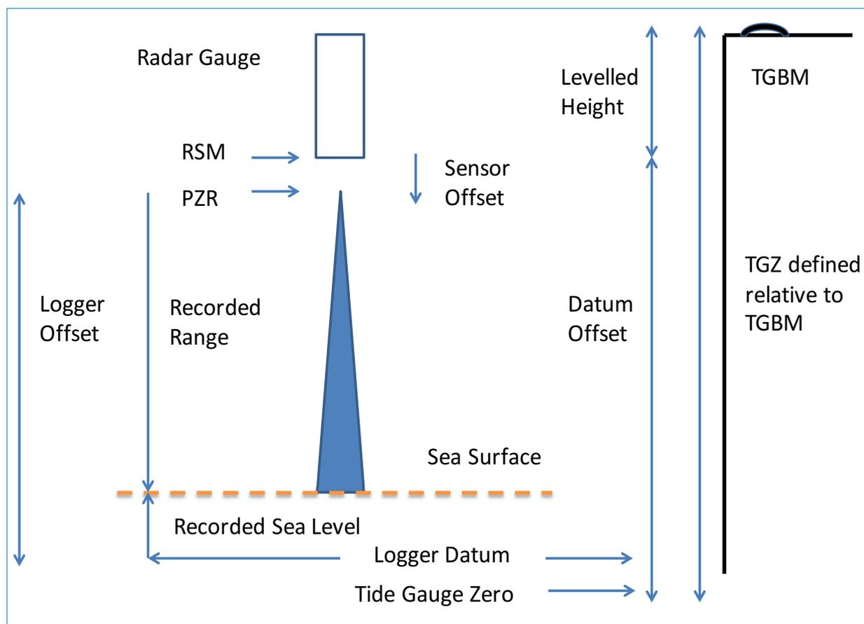
**Figure 4.8** Schematic of a radar gauge, the Reference Survey Mark (RSM) on its casing, its Point of Zero Range (PZR), Logger Datum, Tide Gauge Zero (TGZ), and the Tide Gauge Benchmark (TGBM). All of these levels must be known relative to each other.
