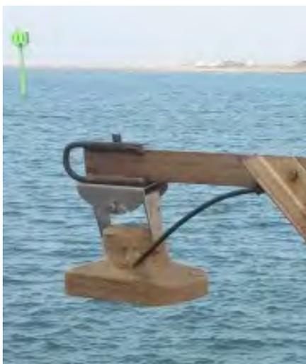
**Figure 3.** Transducers coated in Denso Tape.
