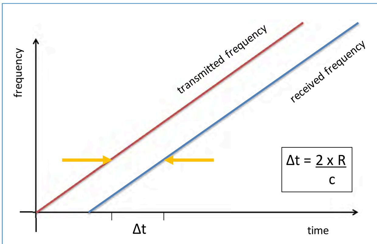
**Figure 2.1** The principle of FMCW measurement with the time difference  $\Delta t$  between the same transmitted and received frequencies increasing in proportion to the distance to the target  $R$ , where  $c$  is the speed of light in air.
