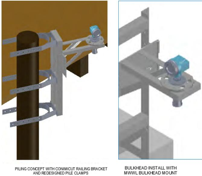
**Figure 4.5** The NOAA flat metal mounting plate with triangular brackets on each side that enable convenient attachment to different types of structure (e.g. piling and bulkhead mountings in this case).
