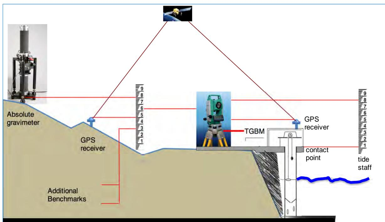
**Figure 6.1** A schematic description of a tide gauge station together with a GNSS receiver for determination of the ellipsoidal height of the sea level measured by the gauge and for the monitoring of vertical land movements. Land movements are also shown being monitored in this figure with the use of an Absolute Gravity meter.
