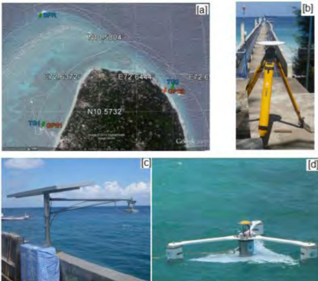
**Figure 7.** [a] Experimental setup and instruments deployed during the Cal/Val experiment at Kavaratti (1-5 October 2012). [b] GPS Base station, [c] Radar gauge (TG2) and [d] GPS buoy (GPS2) deployed at NIOT jetty.
