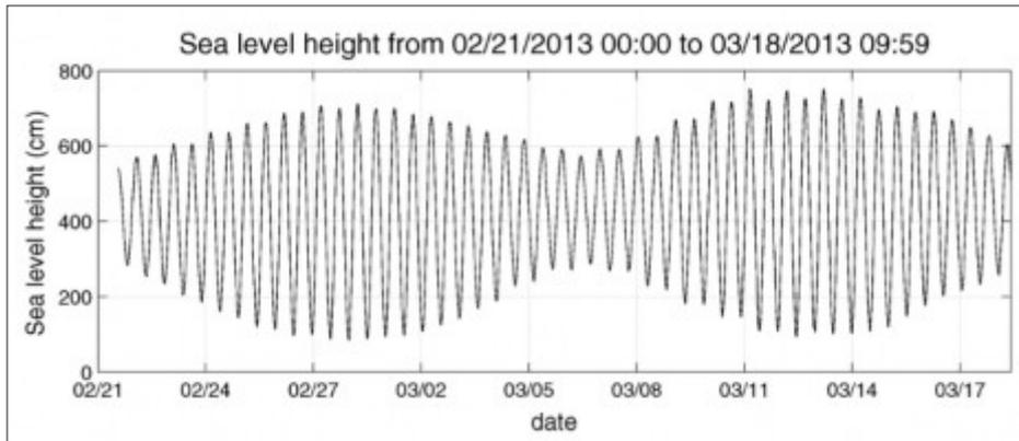
Figure 6. Sea level heights measured with the BM100 radar sensor.
