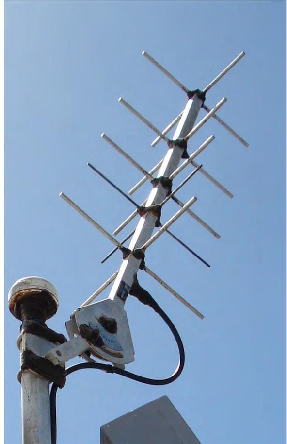
**Figure 7.8** A GOES Yagi antenna. The small hemisphere on the top of the support post is a GPS antenna for time control. (Photograph NOC).
