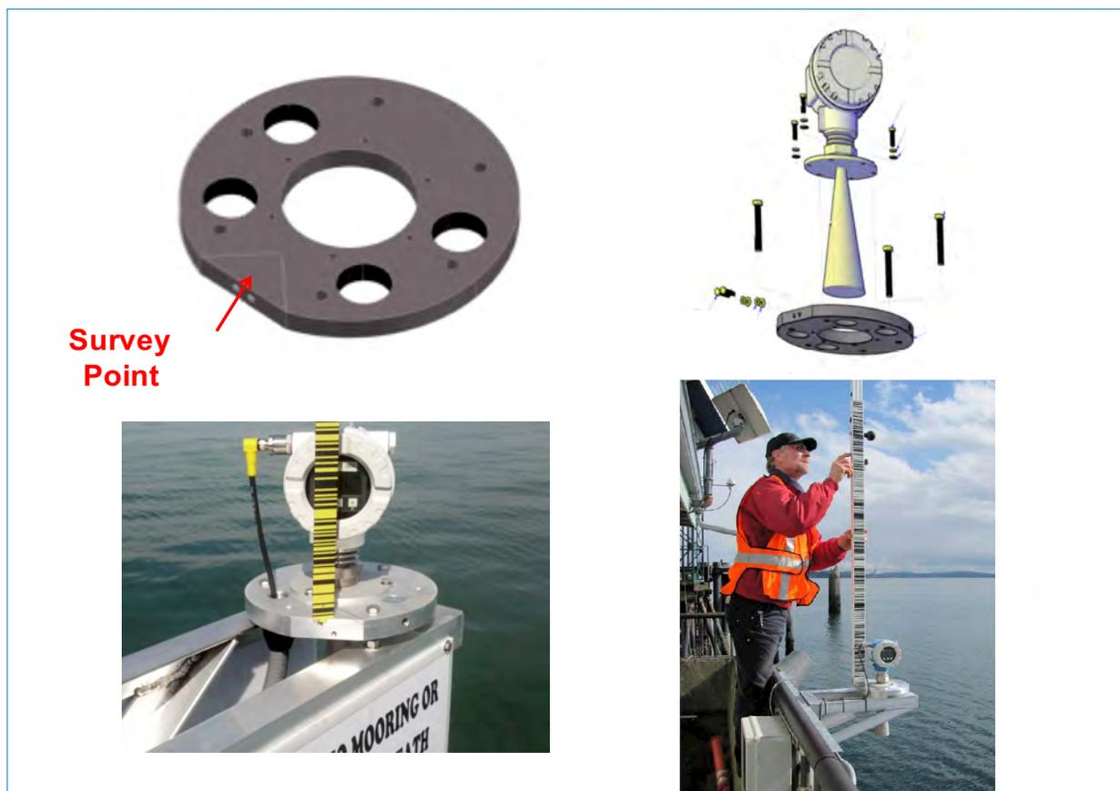
**Figure 4.4** The mounting collar used by NOAA for horn radar gauges such as the Waterlog H-3611. The collar is a 1-inch thick disk of aluminium with holes for attachment of the sensor to the collar and of the collar to the supporting frame. A levelling rod can be placed on an area on the top face of the collar to enable geodetic connection to neighbouring benchmarks. (Photographs NOAA).
