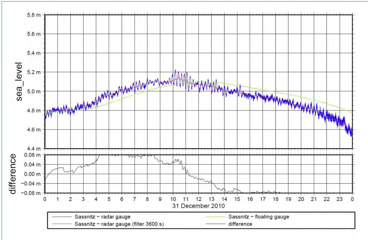
**Figure 7** Comparison of the measured values of the radar gauge with those of the official floating gauge in Sassnitz, representation of the phase delay in the measurement values of both gauges.
