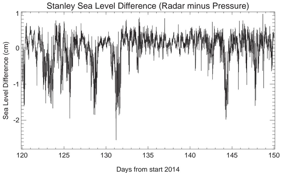
**Figure 5.** Differences between 15-minute values of sea level measured by the H-3611 radar and pressure gauges at Stanley during May 2014. There were several short periods of negative bias in the radar during winter months.
