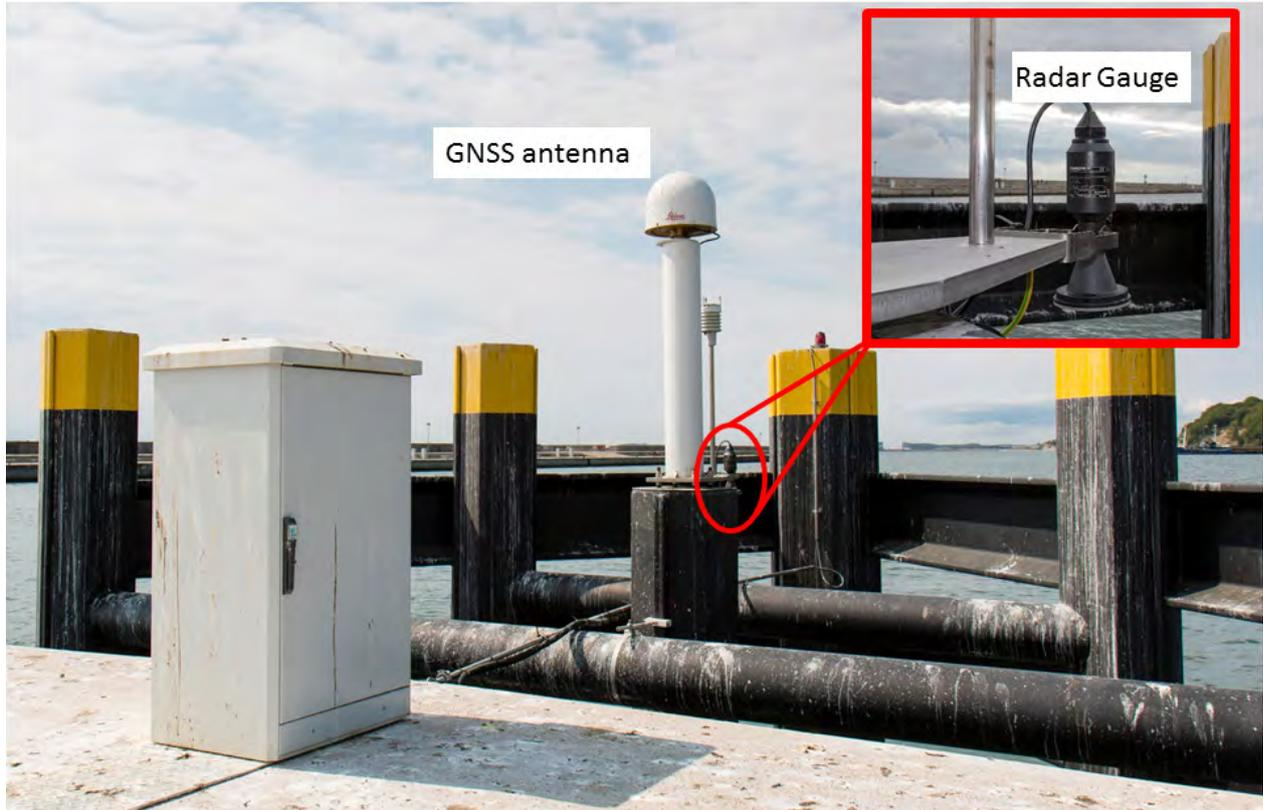
**Figure 12** New GNSS reference station in Sassnitz (GREF station SAS2) with GNSS antenna on top of the antenna pillar, control unit, weather measurement unit and Radar Gauge (in operation since April 2016).
