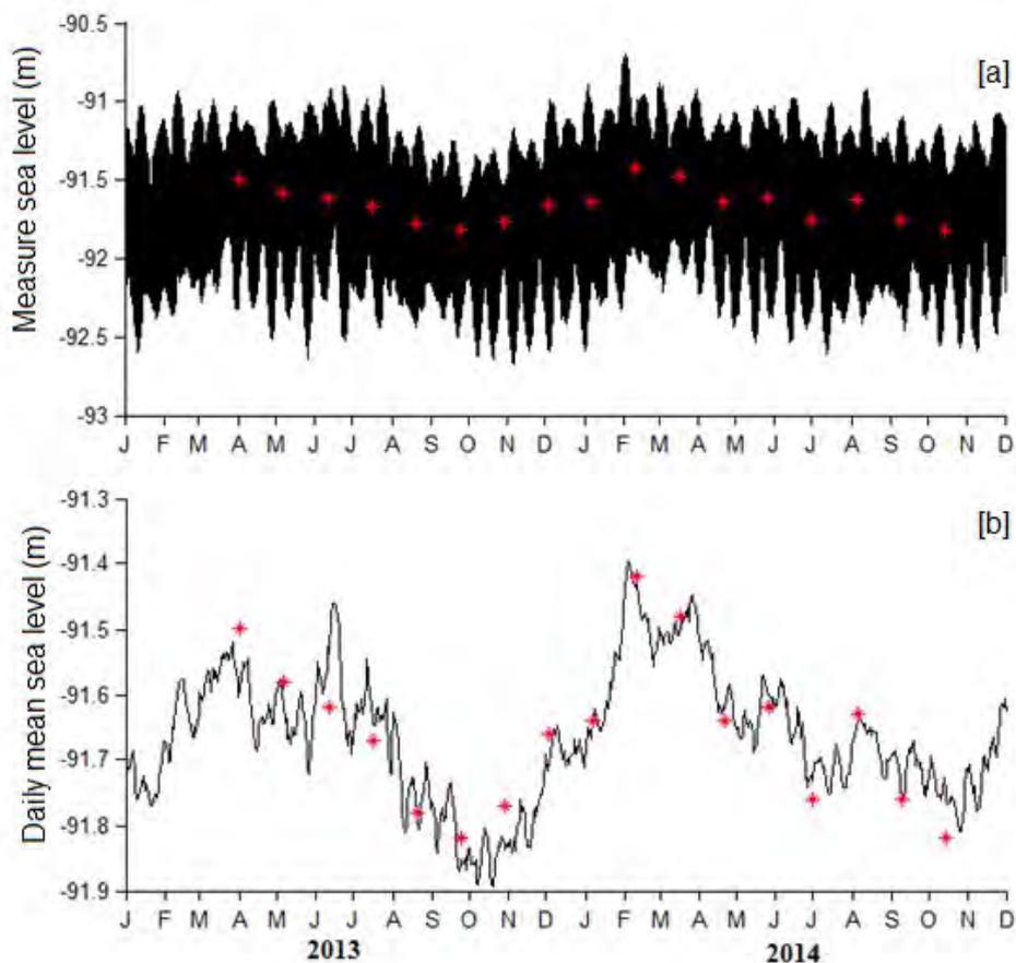
**Figure 9.** [a] Sea-level at 5-minutes interval and [b] Daily-mean sea level data from radar gauge (black line) and sea surface height from Saral-Altika altimeter (red stars) with reference to ellipsoid at Kavaratti [Time is in GMT].
