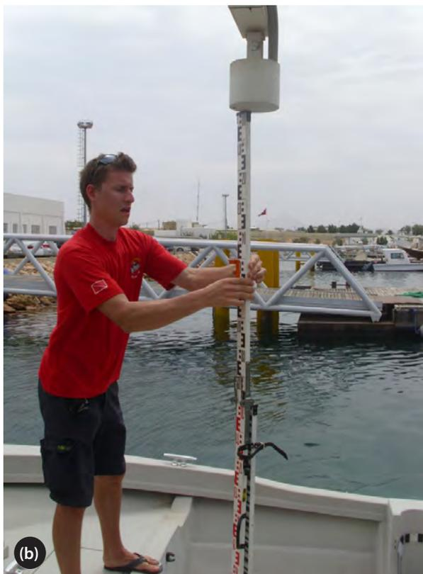
(b) An unusual type of levelling of a radar gauge at Sur in the Sultanate of Oman using a boat in calm conditions. (Photograph T. Schöne, GFZ).
