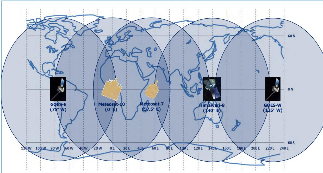
**Figure 7.1** Coverage of the two NOAA GOES satellites over the Pacific and Atlantic, the two EUMETSAT METEOSAT satellites over the Atlantic and Indian Oceans, and JMA Himawari-8 over the Pacific. With regard to METEOSAT, this figure shows the situation as of 2016 with METEOSAT-7 at 57.5°E. This is planned to be replaced by METEOSAT-8 in 2017. (Figure from Sean Burns, EUMETSAT).
