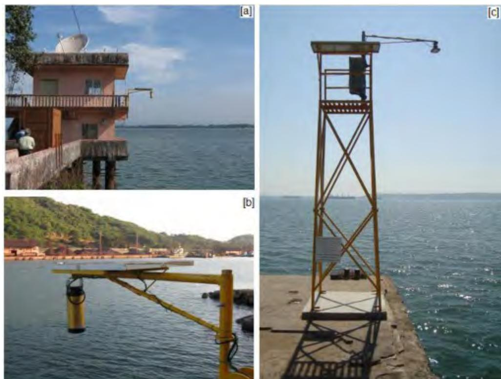
**Figure 3.** Typical installations of microwave based radar gauges at [a] Karwar, [b] Port Blair and [c] Dona Paula.
