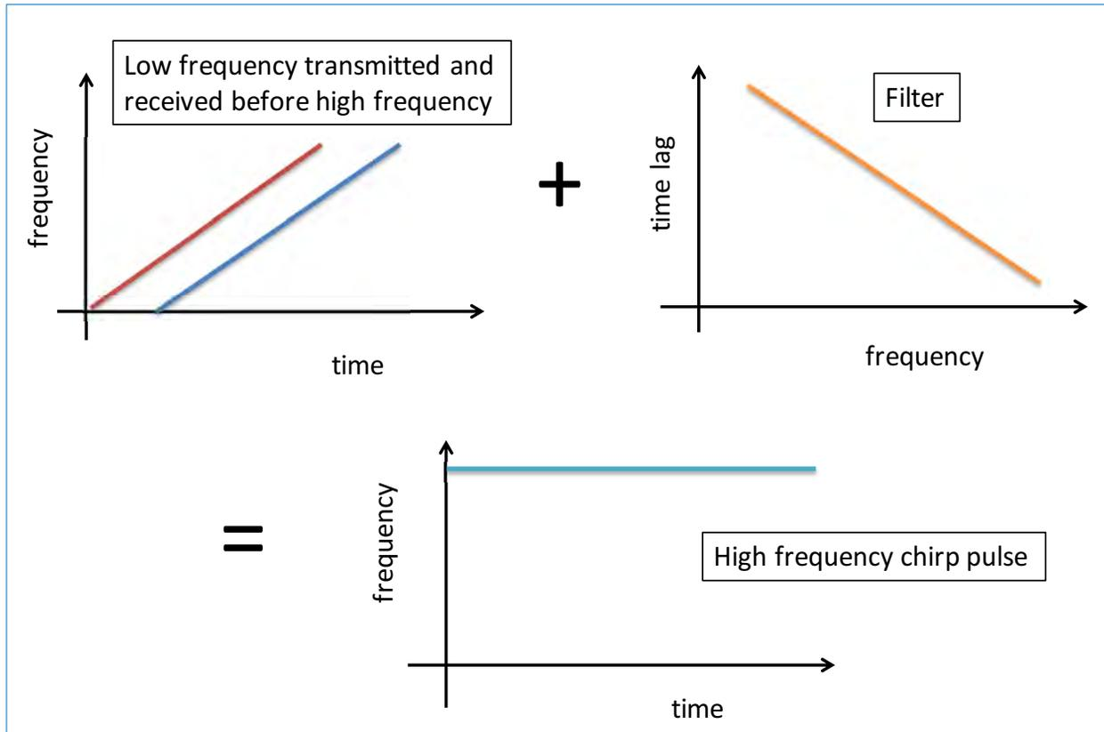
**Figure 2.3** A schematic description of chirp pulse compression. Lower frequency waves are transmitted to, and received back from, the target before the higher frequency waves. A filter is applied to the received signals such that the earlier, lower frequency waves are delayed relative to the later, higher frequency waves. The result is compression of energy into a high frequency 'chirp pulse' packet.
