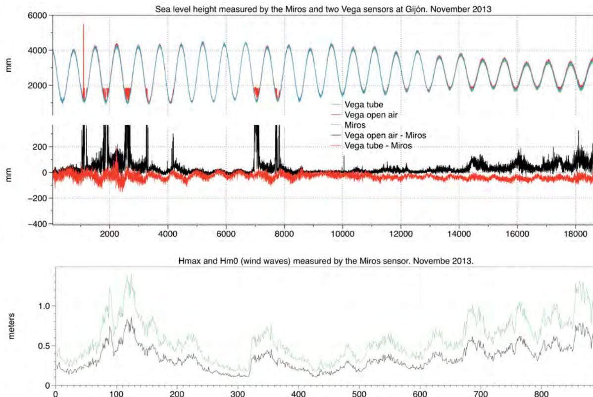
**Figure 3.** Top panel: 1-min sea level data measured by the three sensors (Miros, Vega inside a tube and Vega in the open air) at Gijón harbor, for 14-27 November 2013; medium panel: evolution of the differences between the two Vega sensors and the Miros sensor for the same period; bottom panel: Hmax (green) and Hm0 (black) recorded by the Miros sensor for the same period.
