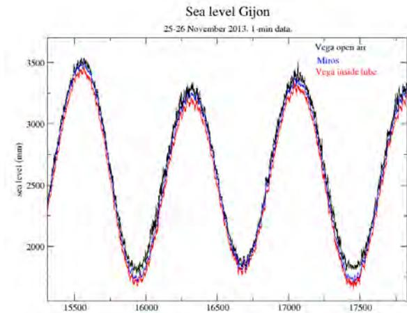
**Figure 4.** Zoom of 1-min sea level data for the two Vega radar sensors installed in Gijón in November 2013 and the permanent Miros sensor.
