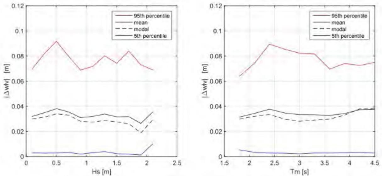
**Figure 11.** Influence of sea state near Borkum on the deviation between water level measurements with a radar array and a float in a stilling well: effect of significant wave height (left) and effect of mean wave period (right).
