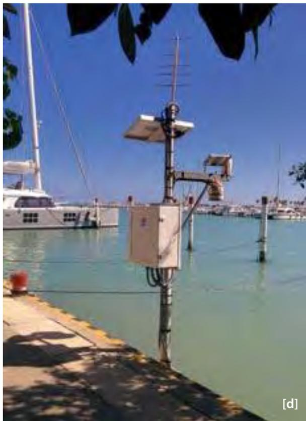
**Figure 2 [d].** Punta Cana sea level station operated by the University of Hawaii Sea Level Center (UHSLC) with the National Office for Meteorology in the Dominican Republic (ONAMET). This single radar configuration is similar to that used by UHSLC at this as well as 9 other stations in the Caribbean and Adjacent Regions (Photo Credit: Nikolai Turetsky, UHSLC)
