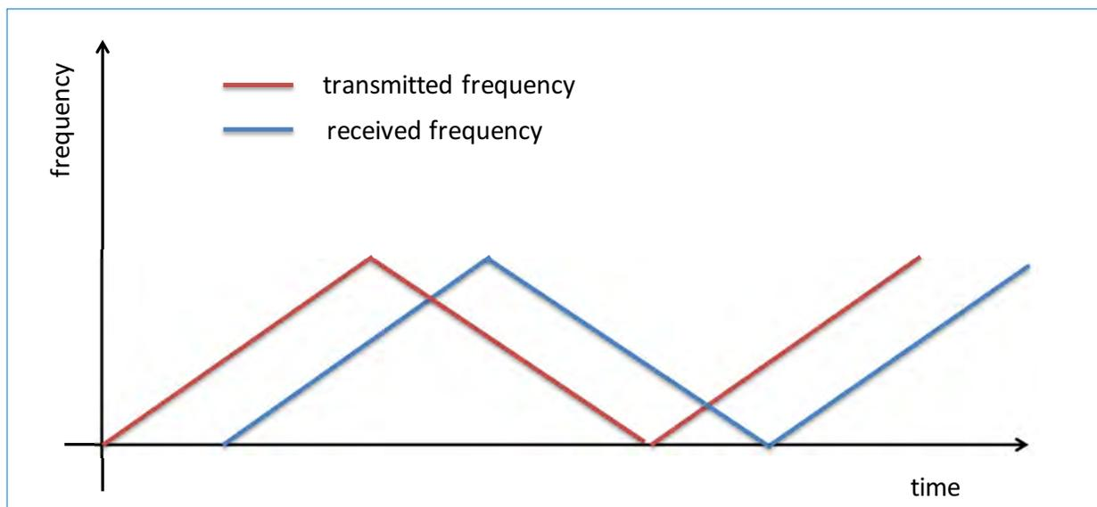
**Figure 2.2** Triangular modulation of frequency used in an FMCW radar gauge.
