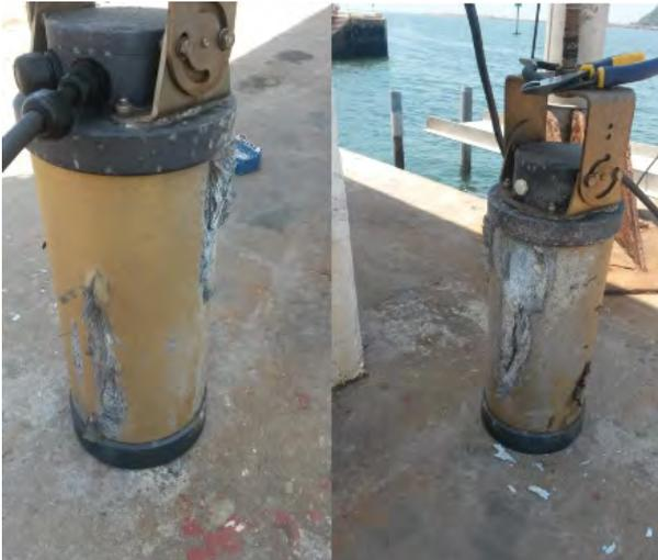
**Figure 2.** Durban's transducer showing corrosion damage.
