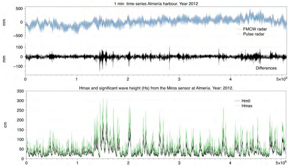
**Figure 9.** Top: 1-min data from both tide gauges and their differences for year 2012; bottom: simultaneous wind wave parameters ( $H_{max}$  and  $H_s$ ) as measured by the Miro sensor for this year.
