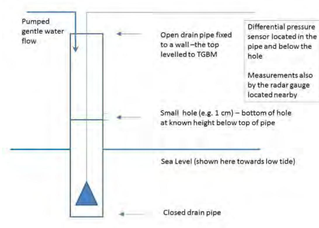
**Figure 4.** Schematic of the 'dribbler gauge' used to determine the effective datum of the H-3611 radar sensor.
