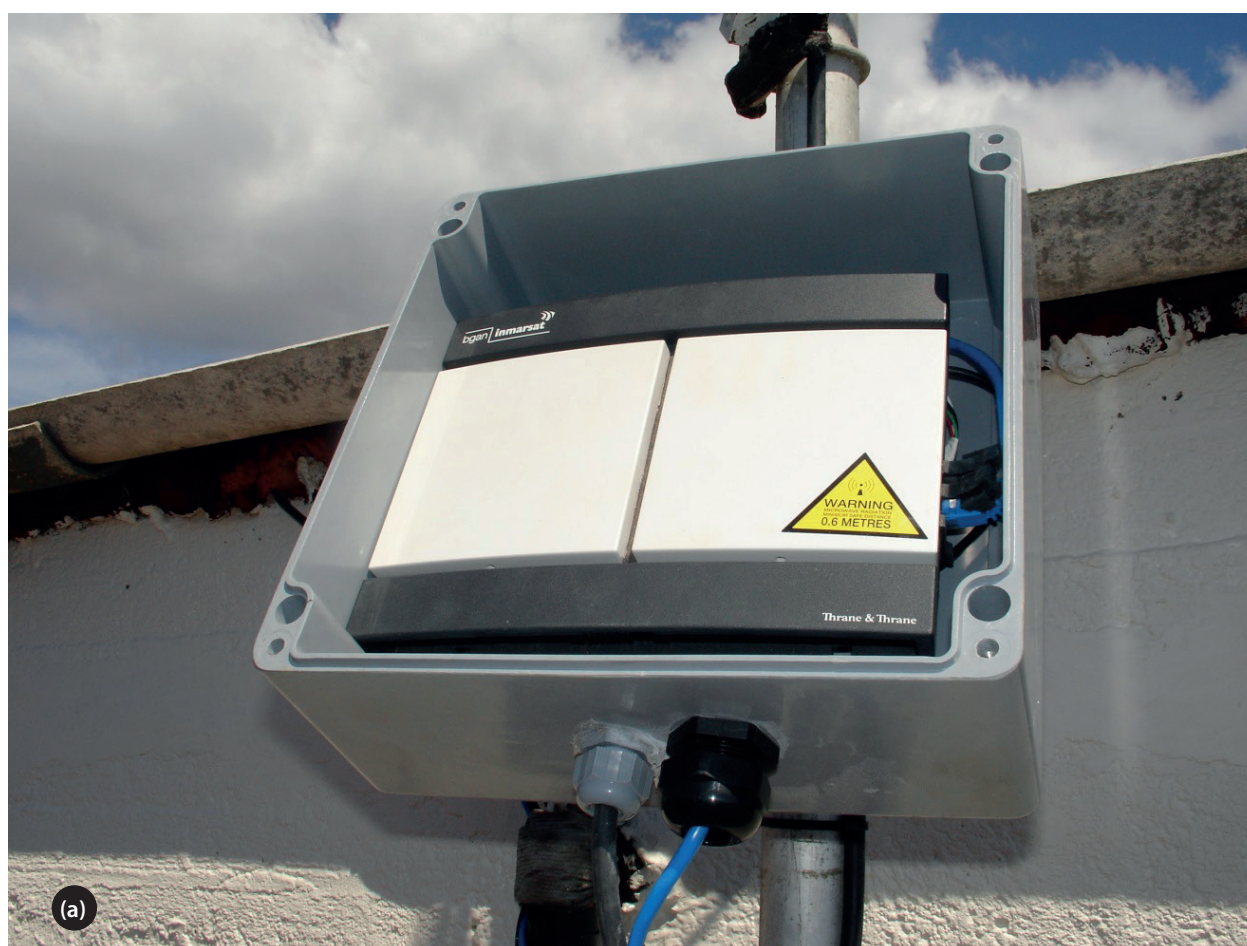
Figure 7.9 (a) Un terminal BGAN Thrane & Thrane Explorer 300 BGAN. (Photo NOC.)
